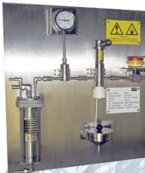
Panel mounted In-Line sample valve with In-Line heat exchanger to cool process media prior to it arriving at the sample valve, and temperature gauge.
