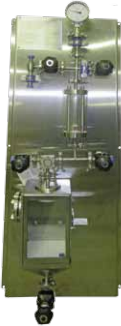
Free standing vessel sampling system for sampling unstable process liquids with self-draining, zero crevice design, and an eductor to generate vacuum.
