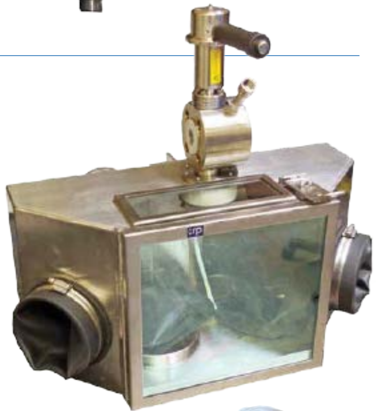
Cabinet with glove ports and padlockable latch
